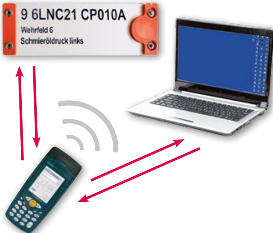
RFID technology and the FP memo sign system facilitate IT-based mobile maintenance and inspection of plants and plant components, pipelines and cables, networks and facilities.
